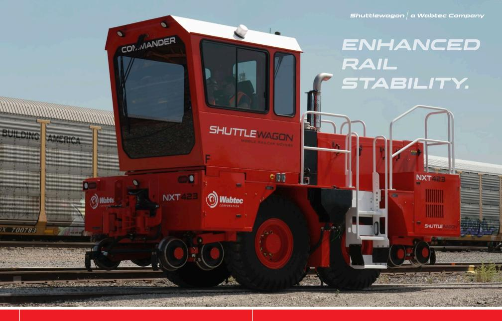
16-inch rail wheels for handling tighter curves
