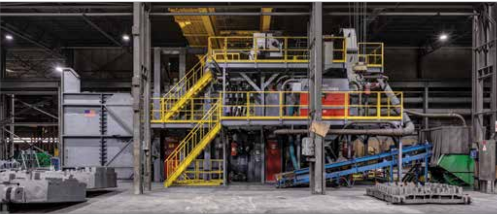
This 28 ft. diameter, 60,000 lb. capacity machine is one of our largest custom solutions in North America. This system with it's main blast zone constructed of 1/2" manganese steel showcases the typical BCT approach with stairway access, floor mounted separation and platforms allowing easy access to all blast wheels .
