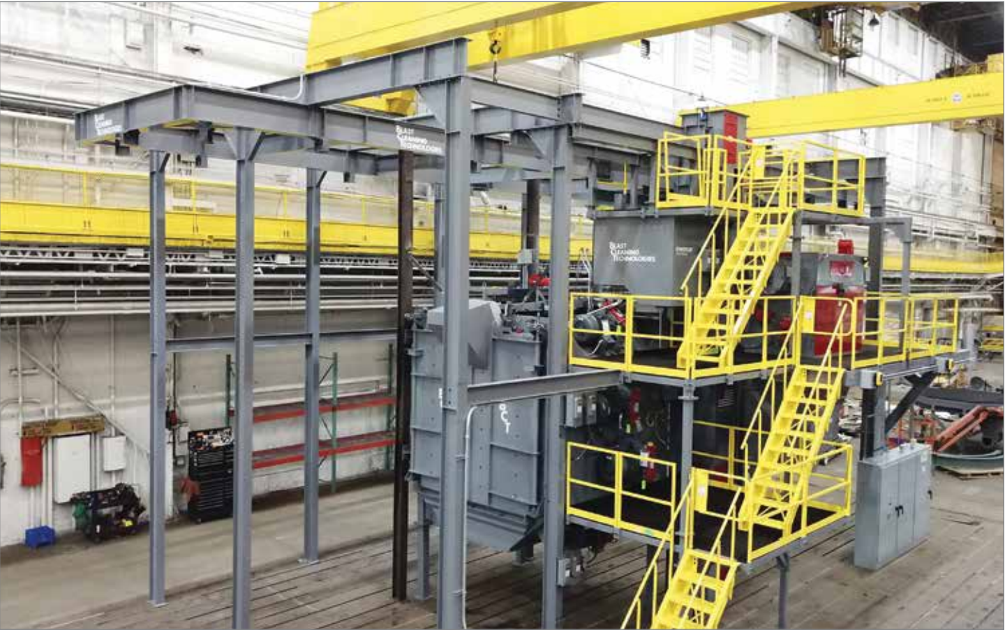
This 28 ft. diameter, 60,000 lb. capacity machine is one of our largest custom solutions in North America. This system with it's main blast zone constructed of 1/2" manganese steel showcases the typical BCT approach with stairway access, floor mounted separation and platforms allowing easy access to all blast wheels .
