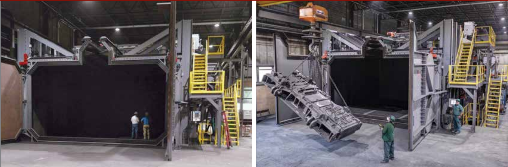
This 28 ft. diameter, 60,000 lb. capacity machine is one of our largest custom solutions in North America. This system with it's main blast zone constructed of 1/2" manganese steel showcases the typical BCT approach with stairway access, floor mounted separation and platforms allowing easy access to all blast wheels .
