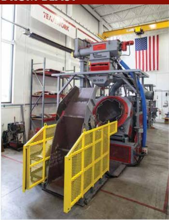
BCT's innovative Drum Blast designs eliminate pinch points while greatly reducing parts damage. Available in 8D, 10D, 12D, 14D, 18D, 30D, 40D and 50D.
